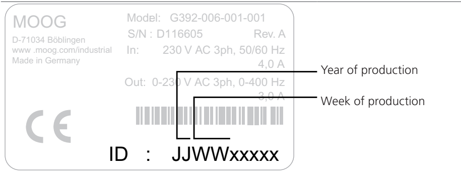
Figure 2.1 MSD Servo Drive rating plate
